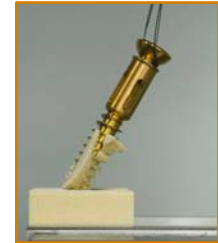
Post-test view of Integrity-SI Fastener (UnifiMI/) test
