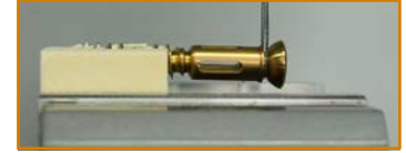
LEFT - Pre-test view of Integrity-SI Fastener (UnifiMI) test setup
