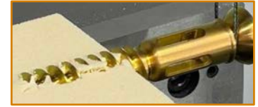
LEFT - Close-up view of UnifiMI threads and the preserved foam between the threads; RIGHT - Close-up view of the buttress threads and associated foam damage
