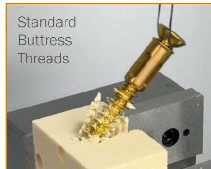
Standard Buttress Threads Integrity screw with buttress threads - very little bone foam still attached to implant
