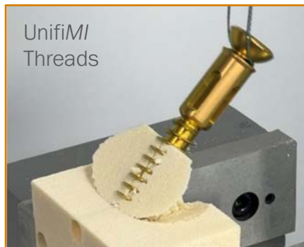
UnifiMI Threads Integrity fastener with UnifiMI threads - bone foam still attached to the implant
