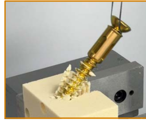
Integrity screw with buttress threads - very little bone foam still attached to implant
