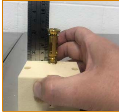
Example test specimen and level of insertion into the bone block
