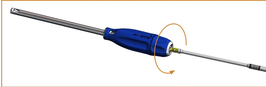
Direction of insertion: central shaft and Blade into Blade-X - opposite direction for removal.
