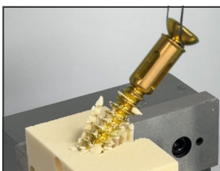
Integrity screw with Buttress threads - very little bone foam still attached to implant
