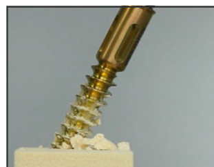
Post-test view of Integrity-SI Screw (Buttress) test
