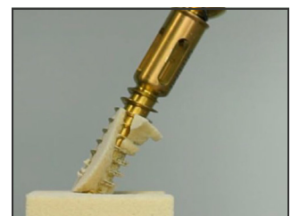
Post-test view of Integrity-SI Fastener (UnifiMI) test
