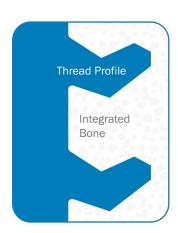
Unique thread geometry instantly and circumferentially interlocks with bone by entrapping and containing bone between the thread form.
