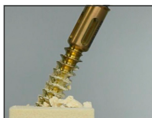
Post-test view of Integrity-SI Screw (Buttress) test
