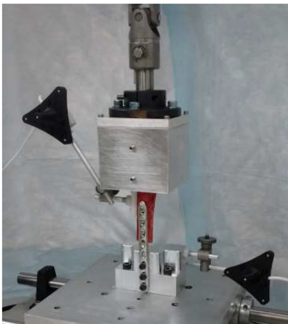
Fig. 2. Experimental set-up for mechanical evaluation of the fracture fixation constructs. PBS soaked towels have been removed for clarity. The fracture fixation plate was fixed to an aluminum block attached to the base of the test machine. The tibial fragment was secured to a universal joint attached to the loading actuator with the bone centerline coaxial to the test machine actuator. Data from the motion tracker sensors (black triangular objects) was used to verify actuator rotary motion during testing.
