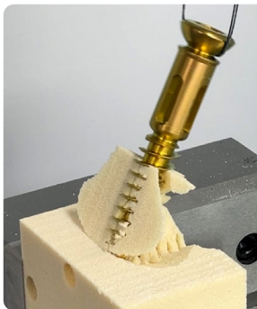
Integrity fastener with UnifiMI threads - bone foam still attached to the implant
