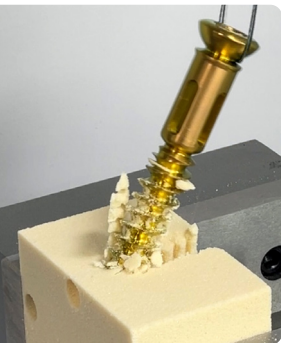
Integrity screw with buttress threads - very little bone foam still attached to implant
