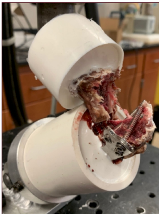
FIGURE 7 Photograph of fracture of the proximal tibial segment through the screw holes.
