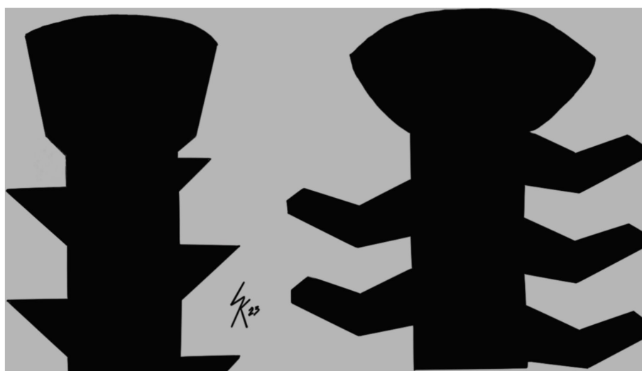
FIGURE 1 Illustration of thread geometry. Left is a locking buttress screw. Right is a bone-screw-fastener.
