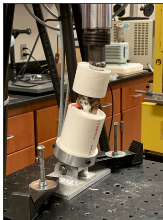
FIGURE 2 Setup for mechanical testing. Truncated and embedded specimen (left tibia) in testing apparatus at 75° to the horizontal. Load introduction via metal sphere proximally. Metal rod and sleeve bearings distally to prevent rotation.
