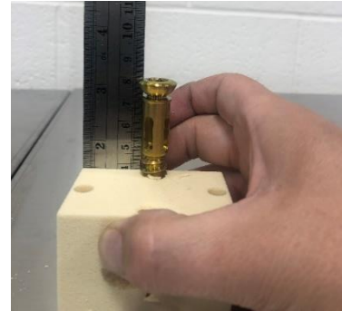
Figure 4 Example test specimen and level of insertion into the bone block
